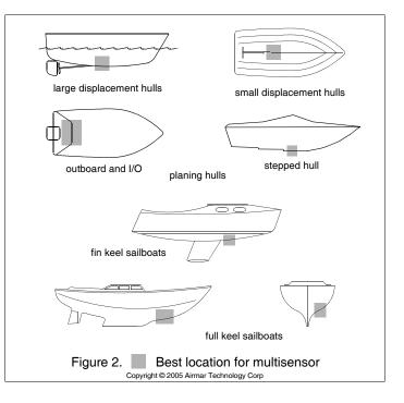
Choose an accessible spot inside the vessel with adequate headroom for the height of the housing, tightening the nuts, and removing the insert. Allow a minimum of 280mm (11").
