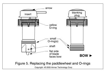
The water lubricated paddlewheel bearings have a life of up to 5 years on low-speed boats [less than 10kn (11MPH)] and 1 year on high-speed vessels. Paddlewheels can fracture and shafts can bend due to impact with water borne objects and mishandling in boat yards. O-rings must be free of abrasions and cuts to ensure a watertight seal. Order a replacement Paddlewheel Kit No. 33-540-01.
