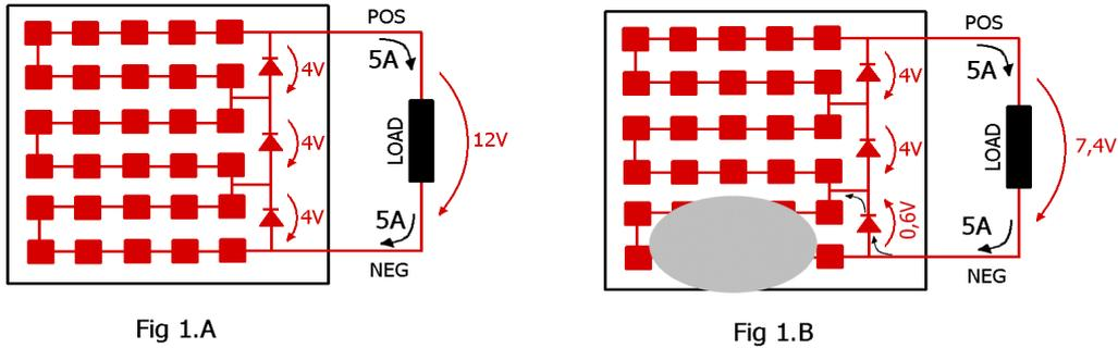
The situation is illustrated in Fig.1.B. The shaded cells can be considered as open circuits. The panel continues to operate but with a lower output voltage of 7.4 V in this case. If this panel is connected in series with other panels, there will be no problem. By contrast, we do not want to connect this panel in parallel with other 12V panels. In Fig.2, I represent the mounting of the
